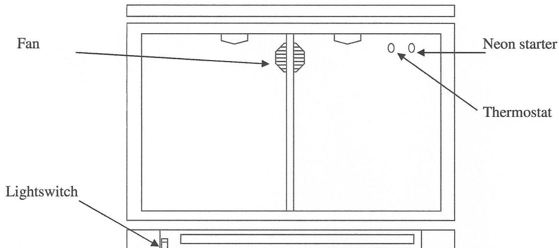
The thermostat can be adjusted with a scale of 1-6, which is equivalent to approximately 2-12°C
