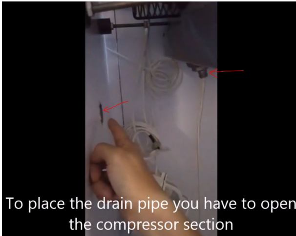
To place the drain pipe you have to open the compressor section
